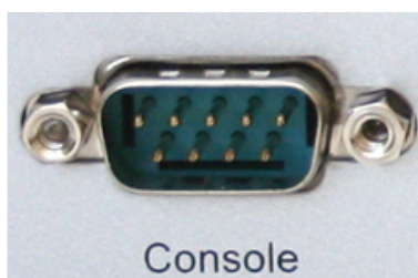
Figure 2.1. The SG50 Series RS-232 Console Port
