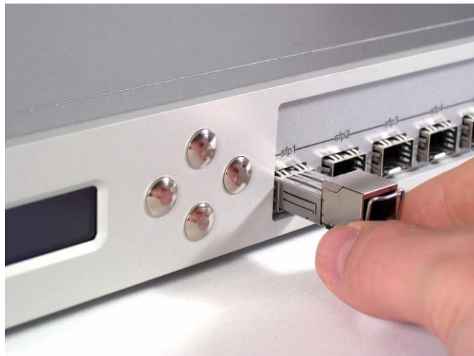
Figure 2.4. Installing a 1000 Base TX module
