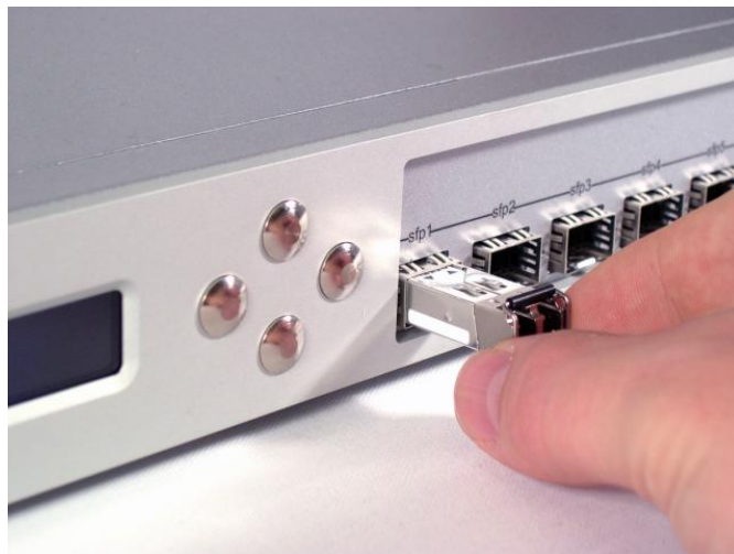
Figure 2.2. Installing a 1000 Base LX/SX module
