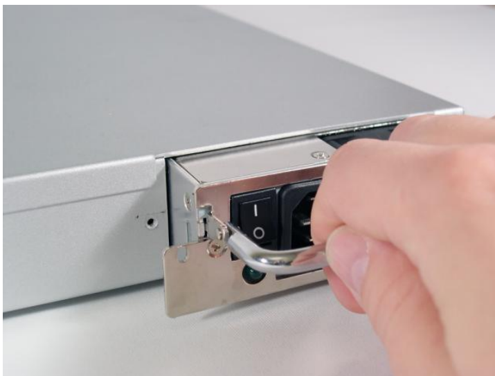
Figure 4.2. Replacing a SG4200 Series power supply.
