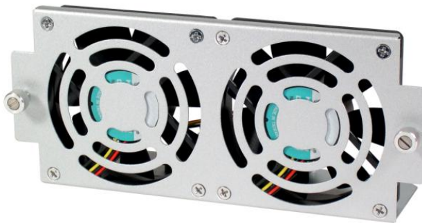
Figure 4.5. An SG4400 Series fan module.
