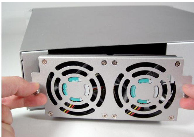
Figure 4.6. Clavister SG4400 Series fan disassembly.
