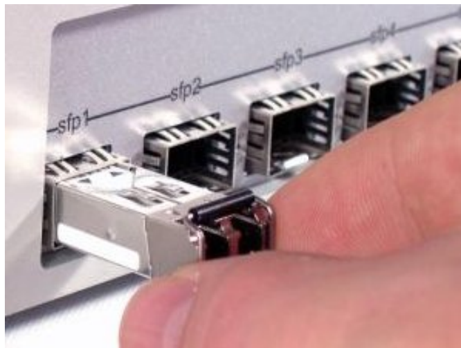
Figure 2.2. Installing a 1000 Base LX/SX module
