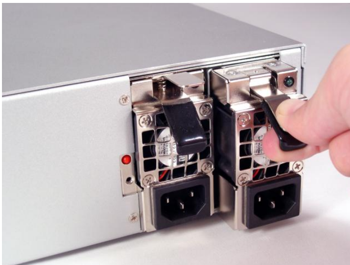
Figure 4.2. Replacing a SG4400 Series power supply.
