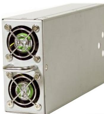
Should a single fan fail in a CFT then the SG5500 Series is able to continue to function for an extended period with that single failure. However the CFT containing the failed fan should be replaced as soon as possible. It is not possible to replace a single fan within a CFT so the whole CFT must be replaced.
