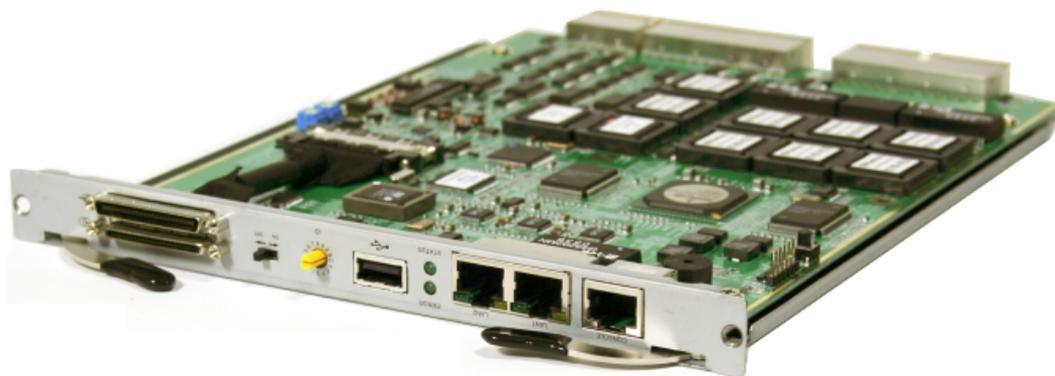
A Chassis Management Module (CMM) provides out-of-band management for the chassis and the Secure Blade Modules. Most configurations require only one CMM per chassis.
