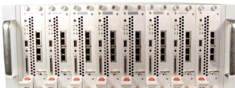
The figure above shows the front of the SG5500 Series chassis with 8 Secure Blade Modules installed:
