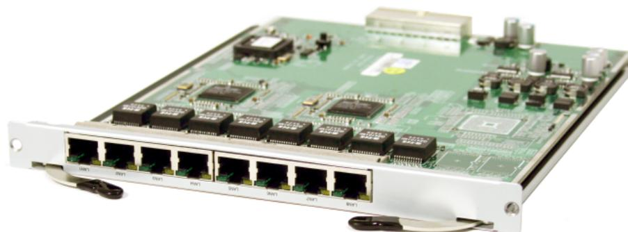
The purpose of the Rear Transition Module (RTM) is to provide additional Ethernet connectivity to the 2 interfaces, **ge1** and **ge2**, on the back of each Secure Blade Module. One port on each RTM is directly connected to one of the physical GE interfaces on the Secure Blade Modules. The upper module connects to all SBM **ge1** interfaces. The lower one connects to all SBM **ge2** interfaces.
