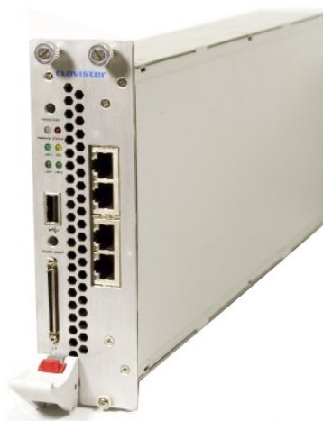
Figure 4.2. A Secure Blade Module (SBM)
