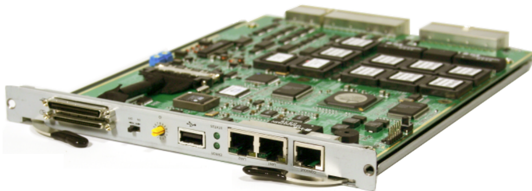
Figure 4.9. A Chassis Management Module (CMM)
